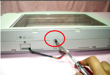
Remove one front fixing screw
