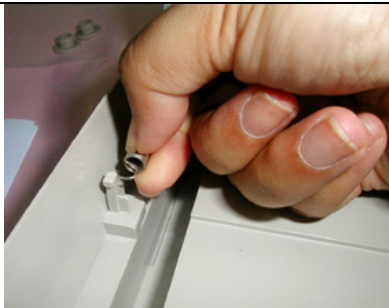
Remove the belt spring from the hinge
