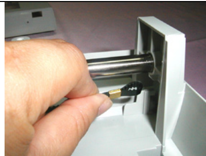
Remove the end of belt from the hinge
