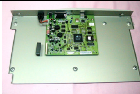
Raise one side of the main board
