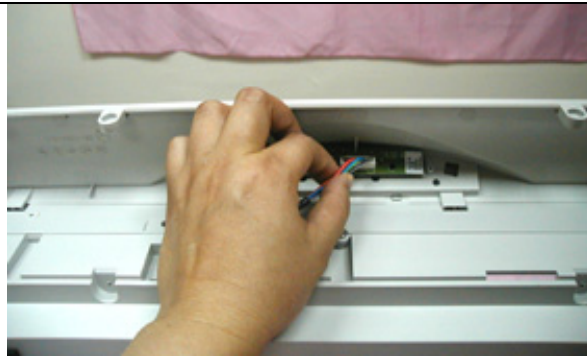
Disconnect the button panel cable
