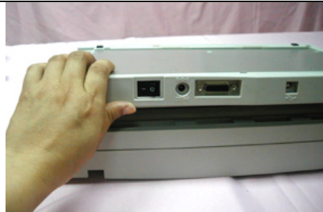
Raise one side of the main board
