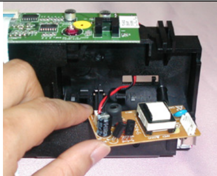
Loosen the inverter from the plastic plate
