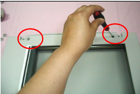
Remove 2 screws beneath the pads
