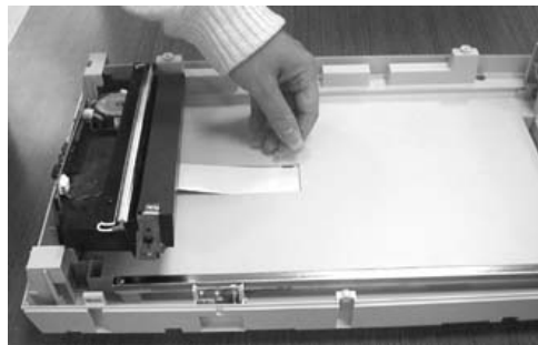
Optical chassis removal
