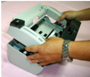
Remove the upper housing
