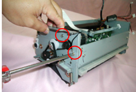
Remove 2 fixing screws
