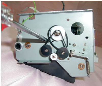
Remove 2 fixing screws on the left external side
