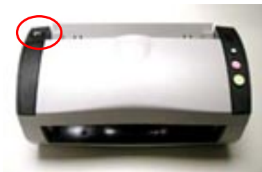
Press the ADF release button
